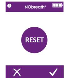
Press and hold the Data Reset button for 5 seconds and the screen will reveal the reset icon.
